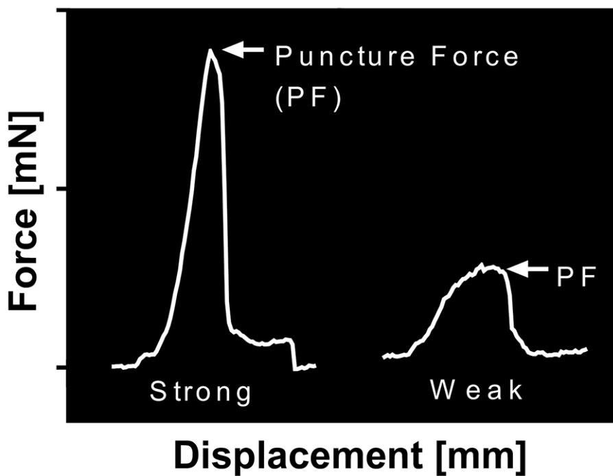
**Fig. S5** Methodology to analyse mechanical properties of the *Avena fatua* coleorhizae by puncture force analysis. Example force-displacement curves for strong and weak coleorhizae. For further details about the device used see Figure 5 in the review 'The biomechanics of seed germination' by Steinbrecher and Leubner-Metzger, *J Exptl Bot* 68:765-783 (2017).
